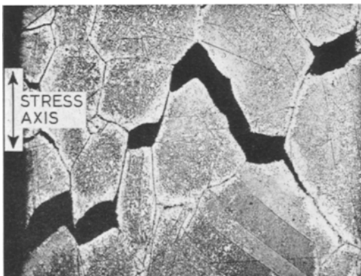
Figure 10 Grain boundary cracks in the surface layer of large-grained specimen strained 27% to fracture at 750^\circ\text{C} ( \times 82 ).
